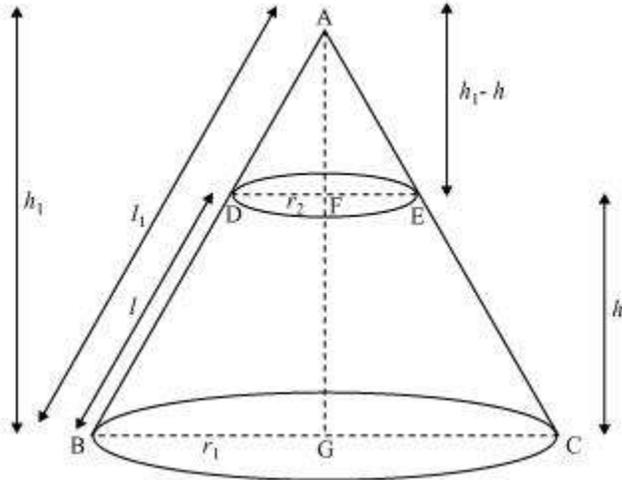
Let ABC be a cone. A frustum DECB is cut by a plane parallel to its base. Let  $r_1$  and  $r_2$  be the radii of the ends of the frustum of the cone and  $h$  be the height of the frustum of the cone.
