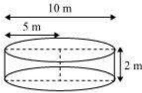
Radius ( $r_2$ ) of circular end of cylindrical tank =  $\frac{10}{2} = 5$  m
