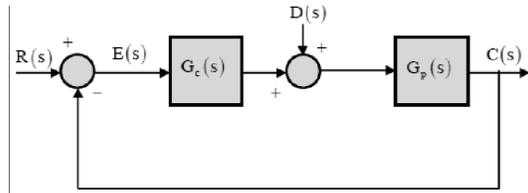
$$G_p(s) = \frac{2.2}{(1+0.1s)(1+0.4s)(1+1.2s)}, G_c(s) = k \left( \frac{1+T_1s}{1+T_2s} \right)$$
