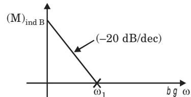
$K = (\omega)^n$  : where  $n$  is no. of poles from the given plot
