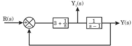
$$\text{Open loop transfer function} = \left[ \frac{(3s + 1)}{s(s-1)} \right]$$
