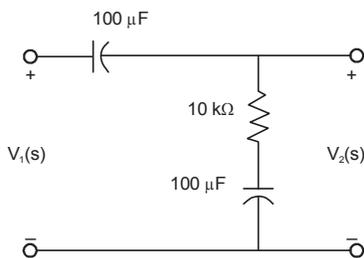
129. Assuming zero initial condition, the response  $y(t)$  of the system given below to a unit step input  $u(t)$  is
