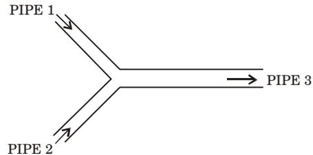
Assuming the water properties and the velocities to be uniform across the cross-section of the inlets and the outlet, the exit velocity (in m/s) in pipe 3 is
