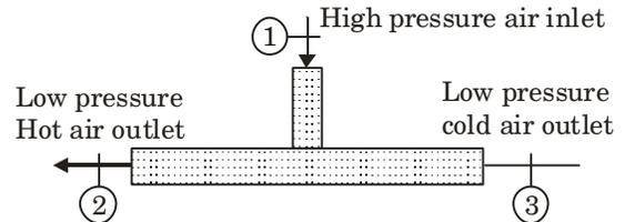
Assume constant specific heat of air is 1005 J/kg.K and gas constant is 287 J/kg.K. There is no work transfer across the boundary of this device. The rate of entropy generation is \_\_\_\_\_ kW/K (round off to one decimal place).
